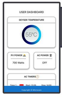
A user dashboard indicates Geyser Temperature, Solar or Grid Power & Timers.
